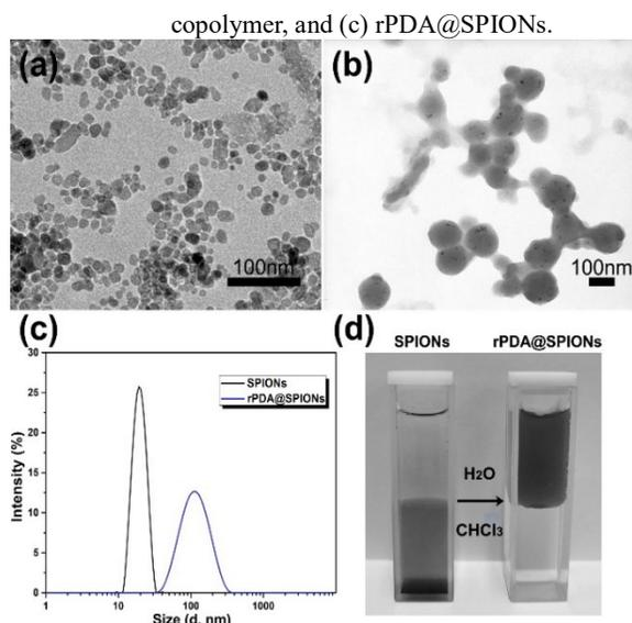
**Fig. 4.** TEM images of (a) oleic acid-coated SPIONs, and (b) after the ligand exchange process (rPDA@SPIONs); (c) DLS data showing the changes of hydrodynamic size (in diameter) of SPIONs before, and after ligand exchange with rPDA crosslinked copolymer; (d) Photograph of oleic acid-coated SPIONs (left) and water-soluble rPDA@SPIONs (right) dispersed in water and chloroform.
