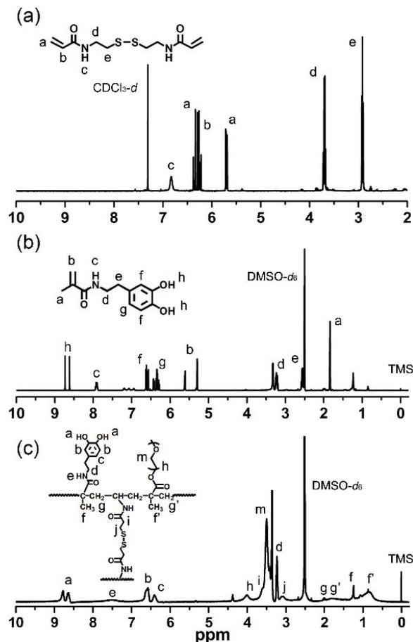
Fig. 2.  $^1\text{H}$  NMR spectra of BACy (a)  $\text{CDCl}_3-d$ , DMA (b) and rPDA crosslinked copolymer (c) in  $\text{DMSO}-d_6$ .
