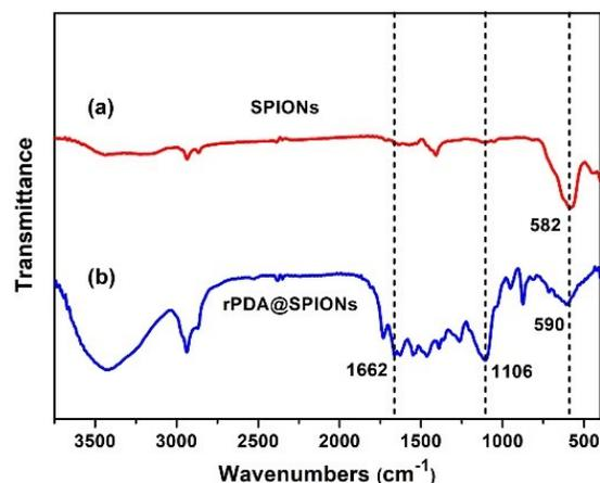
Fig. 3. FTIR spectra of (a) SPIONs, (b) rPDA crosslinked
