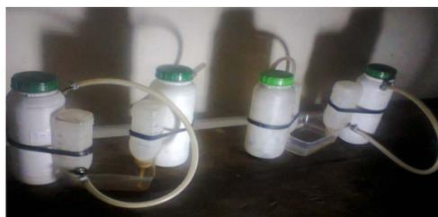
Fig. 1 Experimental setup for biogas production
